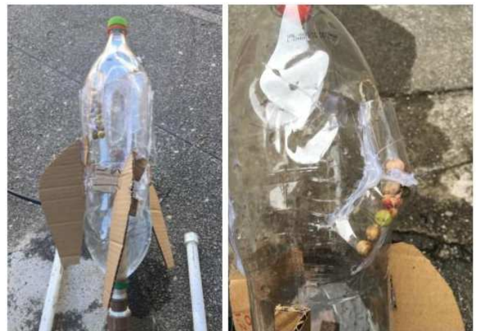
FIGURE 2. Rockets used in the testing phase, based on the OBAFOG level 3 model. On the left, the model with straight tubes, and on the right, the model with curved tubes. A whole PET bottle forms the body and another cut bottle is positioned as the tip of the rocket. Small tubes, made from the remaining part of the cut bottle, store the seeds. The three wings are made of cardboard.
