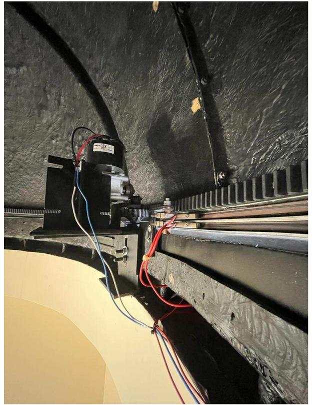
FIGURE 4. Trapdoor rotation motor
