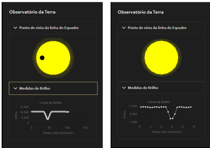
FIGURE 3. Screenshot of the light intensity graphs. In this simulation, the measuring equipment is located on the equator line and the study phenomena consists of the moon’s transit in front of the Sun. Every time the moon passes in front of the Sun, a valley appears in the graph, as the light intensity measured decreases depending on the distances and sizes involved.
